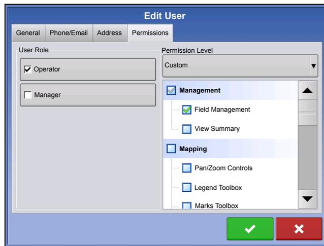
Display uses Traditional mode when Field Management is checked. Events using the Traditional mode are tied to the Grower/Farm/Field structure.
