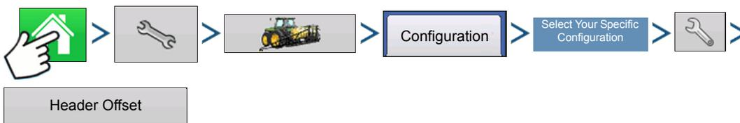
Press: Home button > Setup (wrench) button > Configuration (tractor) button > Configuration tab > your specific configuration > Setup (wrench) button > Header Offset button
