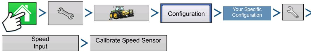
Press: Home button > Setup (wrench) button > Configuration (tractor) button > Configuration tab > your specific configuration > Setup (wrench) button > Speed Input button > Calibrate Speed Sensor
