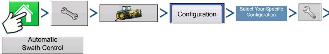
Press: Home button > Setup (wrench) button > Configuration (tractor) button > Configuration tab > select your specific configuration > Setup (wrench) button > Automatic Swath Control button
