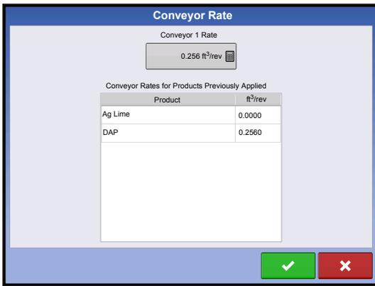
The **Conveyor Rate** button opens a setup screen where the conveyor rate can be inputted and a table of previously applied products and conveyor rates is shown.
