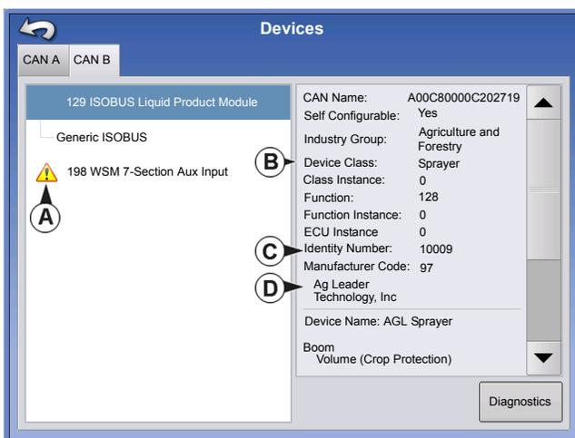
Pressing the Diagnostics button on the Devices screen brings up the ISO Node Diagnostics screen which shows the following information.
