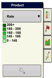
Press the Map Legend button at the top of the Mapping Toolbox, and the Legend appears. User can choose between Rate or Coverage using the drop-down menu.
