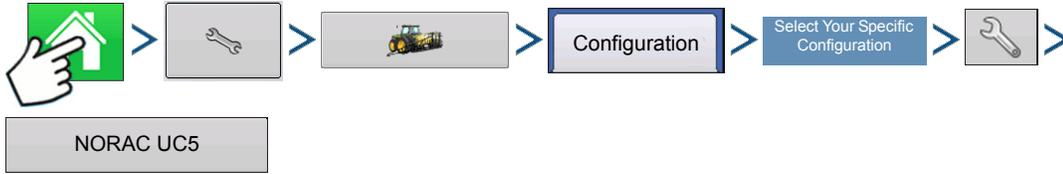
Press: Home > Setup (wrench) button > Configuration (tractor) button > Configuration tab > (*your particular Operating Configuration*) > Setup (wrench) button > NORAC UC5 button
