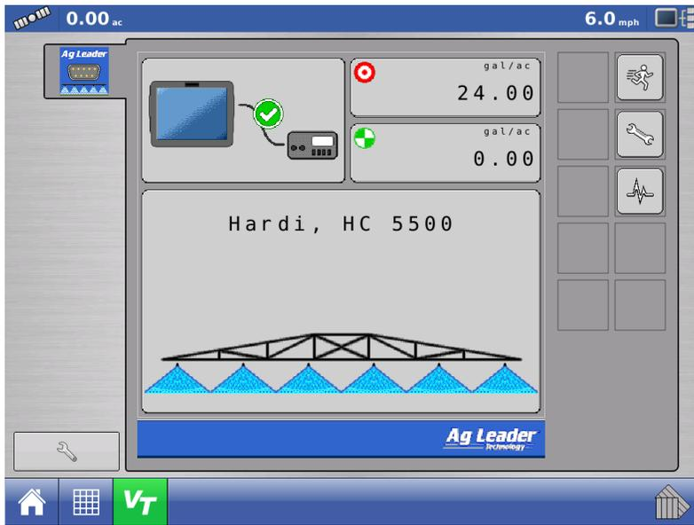
The status screen provides the user with readout of the connected controller's target rate, actual rate, section status, and connection status.
