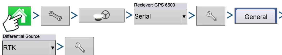
Press: Home button > Setup (wrench) button > GPS button > Serial (from Receiver drop-down box) > Receiver Setup (wrench) button > General tab > RTK (from Differential Correction drop-down box) > Differential Source Setup (wrench) button
