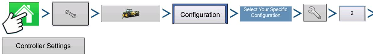
Press: Home button > Setup (wrench) button > Configuration (tractor) button > Configuration tab > your specific configuration > Setup (wrench) button > 2 tab > Controller Settings button
