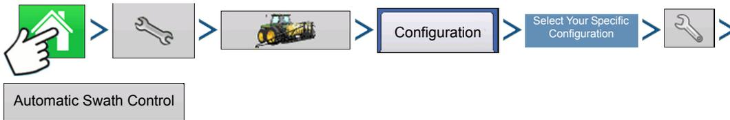
Press: Home button > Setup (wrench) button > Configuration (tractor) button > Configuration tab > your specific configuration > Setup (wrench) button > Automatic Swath Control button
