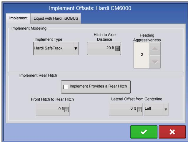
When using Hardi ISOBUS, Implement Modeling can be set to Hardi SafeTrack. This allows display to accurately calculate path of sprayer.
