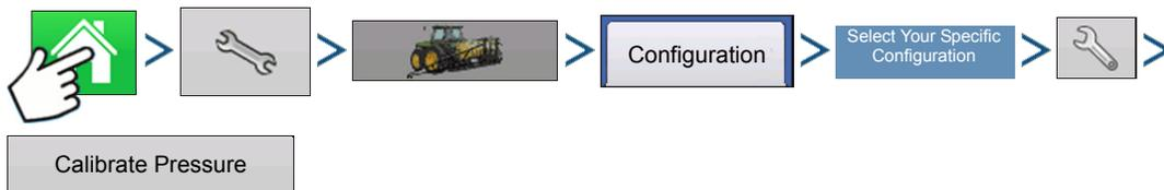
Press: Home button > Setup (wrench) button > Configuration (tractor) button > Configuration tab > select your specific configuration > Setup (wrench) button > Calibrate Pressure button
