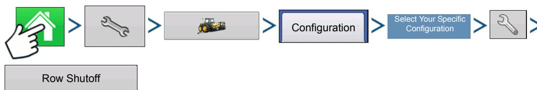
Press: Home button > Setup (wrench) button > Configuration (tractor) button > Configuration tab > your specific configuration > Setup (wrench) button > Row Shutoff button
