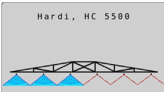
**Boom Section Status** – Indicates the on/off status of the boom sections sent to the connected controller.
