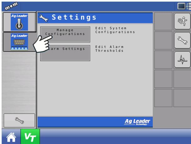
Press Manage Configurations button to edit system configurations.
