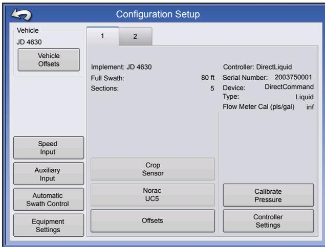
Press: Home button > Setup (wrench) button > Configuration (tractor) button > Configuration tab > your specific configuration > Setup (wrench) button
