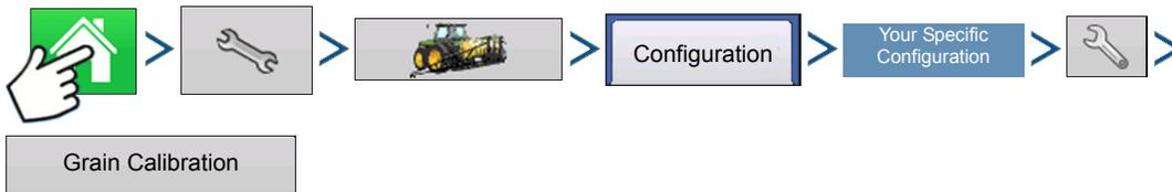
Press: Home button > Setup (wrench) button > Configuration (tractor) button > Configuration tab > your specific configuration > Setup (wrench) button > Grain Calibration button
