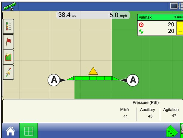
After specifying Fence Row Nozzle settings at the Auxiliary Input Assignment screen, the **Fence Row Nozzle Indicators (A)**, which are shaped like triangles, appear on either side of the sections behind the vehicle icon.
