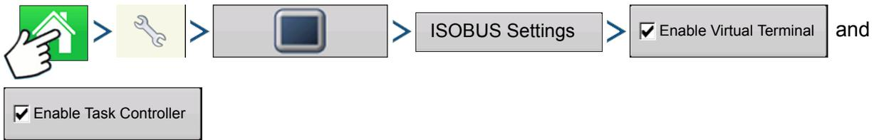
Press: Home button > Setup (wrench) button > Display button > ISOBUS Settings > Enable Virtual Terminal checkbox and Task Controller checkbox
