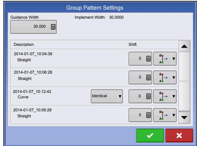
Straight AB, Identical Curve, Adaptive Curve and Pivot Patterns can be grouped. SmartPath cannot be grouped.
