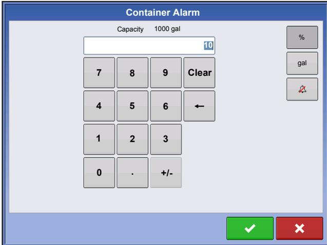
If you wish to adjust your container level warnings, use the following buttons on the right-hand side of the Container Alarm screen to make these adjustments.
