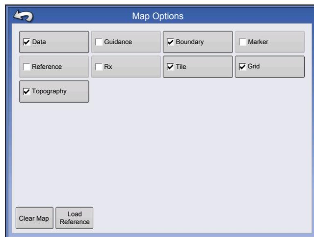
If you have RTK GPS reception, you are allowed to collect an elevation survey. This will allow you to collect the Lat/Long and elevation values as you traverse the field. A point will be dropped every 3 meters as you drive regardless of speed, or direction. If you are collecting during operations like planting or application using autoswath, it will also log points outside the boundary of the field (i.e. through a grassed waterway) to get the most information throughout the field.
