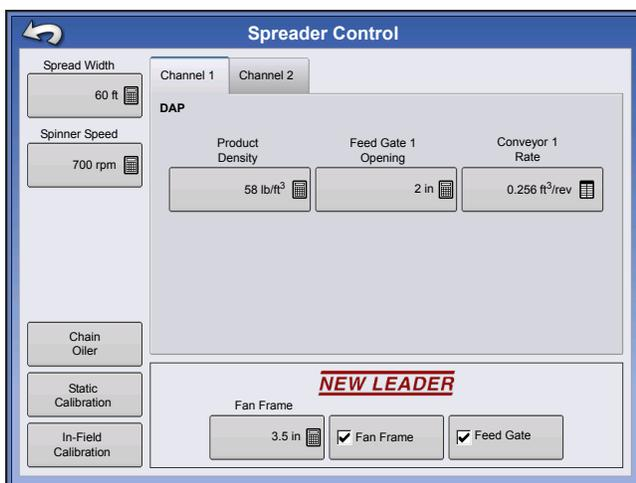
The Spreader Control screen has a tab for each control channel/product being applied. Select the desired channel and press the **Conveyor Rate** button.
