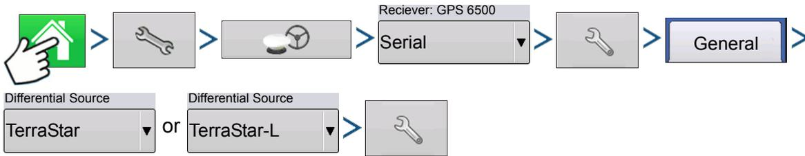
Press: Home button > Setup (wrench) button > GPS button > Serial (from Receiver drop-down box) > Receiver Setup (wrench) button > General tab > TerraStar (from Differential Correction drop-down box) > Differential Source Setup (wrench) button
