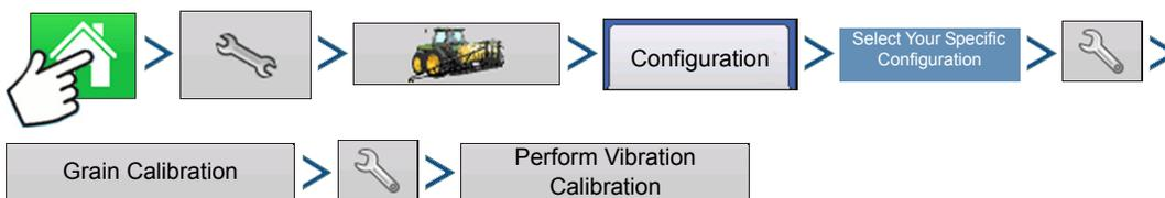
Press: Home button > Setup (wrench) button > Configuration (tractor) button > Configuration tab > your specific configuration > Setup (wrench) button > Grain Calibration button > Setup (wrench) button > Perform Vibration Calibration button
