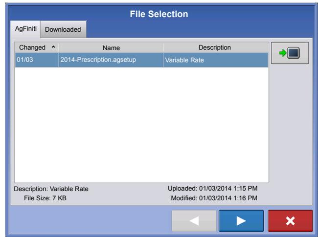
The Downloaded tab shows AgSetup files that are stored on the internal memory of the display. These files can be accessed when there isn't an internet connection, but Wi-Fi adapter must be inserted.
