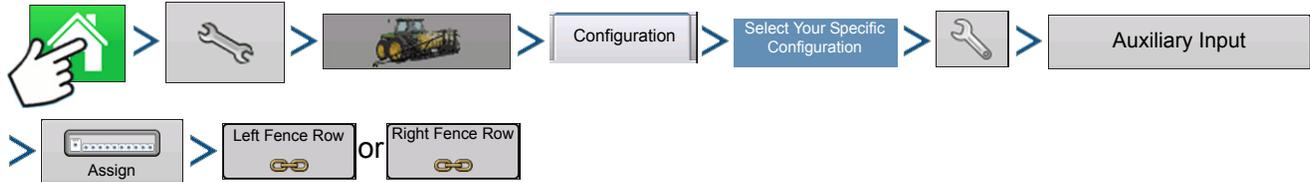
Press: Home button > Setup (wrench) button > Configuration (tractor) button > Configuration tab > select your specific configuration > Setup (wrench) button > Auxiliary Input button > Assign button > Left Fence Row or Right Fence Row. For more information on Auxiliary Input Settings, see [“Auxiliary Input” on page 74](#).
