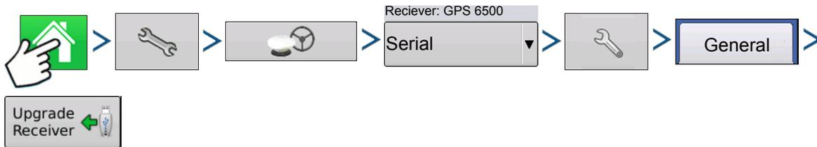
Press: Home button > Setup (wrench) button > GPS button > Serial (from Receiver drop-down box) > Receiver Setup (wrench) button > General tab > Upgrade Receiver button
