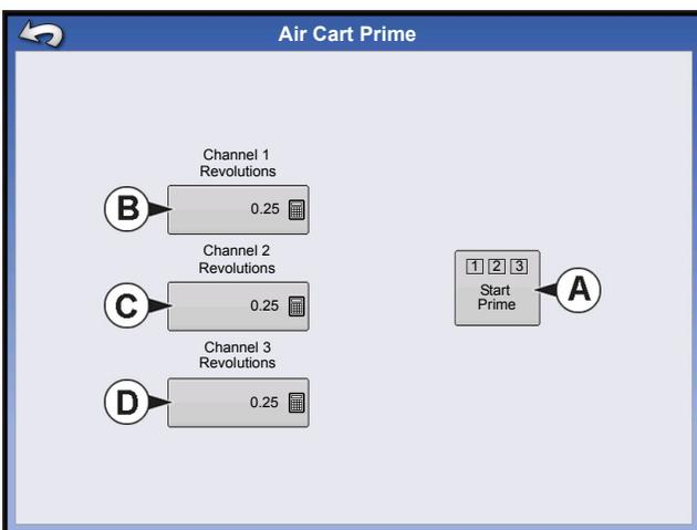
The **Air Cart Prime** screen appears with input buttons for each channel used. The setting determines the revolutions necessary to prime the meter shaft. Settings are independent by channel, and can be entered using .
