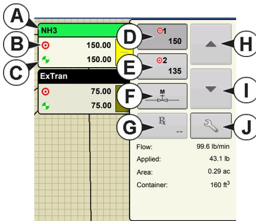
During DirectCommand Run Time operations, the Product Tabs are shown in the upper right-hand side of the Map screen. Press the Product Tabs, and an extended view shows the Rate buttons, Manual Valve Control button, Prescription button, Rate
