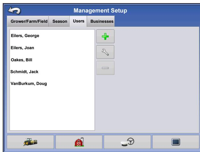
Management Setup screen - User tab allows user to add, modify, or delete users from the display.
