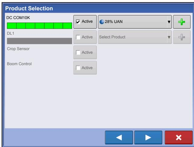
If a configuration is loaded with undetected modules, the Product Selection screen may show some grayed out (unavailable) options. The example to the left shows that the Direct Command module is active but Direct Injection, Crop Sensor, and Boom Control modules are grayed out and not functional.
