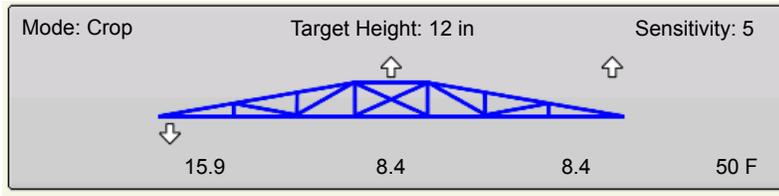
Pressing the **Boom Height Control Options** button (A) opens the **Boom Height Control Options** screen (B). At this screen, you can adjust the boom's Mode, Sensitivity and Target Height.
