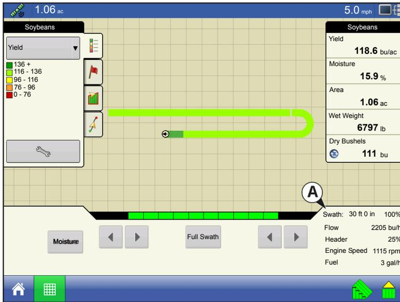
Once an operating configuration is created for a CLAAS Quantimeter harvest configuration, and a field operation configuration is created at the Home screen, you can view map screen data.
