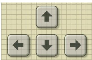
Press the grid area of the Map screen, and four arrow icons appear at the bottom right of the Map screen. An example showing these arrow buttons is at left. Pressing these arrow icons will move the center of the Map screen in the direction of the arrow button.
