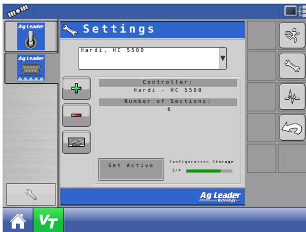
A user can add, remove, edit, or select an active configuration. The module will save up to 4 configurations.
