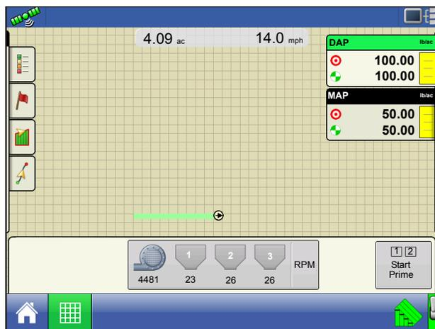
The **Start Prime button (A)** begins the meter prime routine and each meter shaft will rotate the number of revolutions as defined on the Air Cart Prime Screen.
