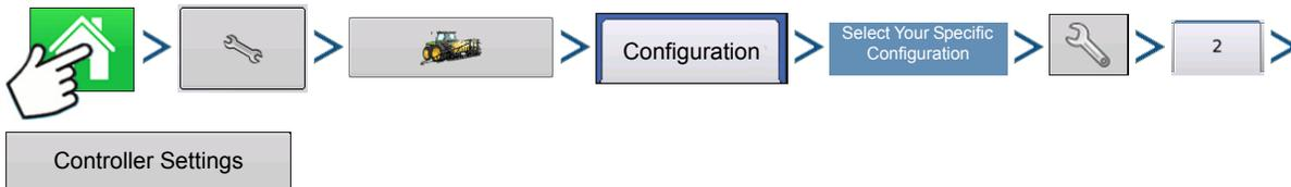
Press: Home button > Setup (wrench) button > Configuration (tractor) button > Configuration tab > your specific configuration > Setup (wrench) button > 2 tab > Controller Settings button
