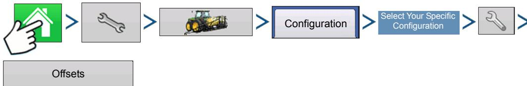
Press: Home button > Setup (wrench) button > Configuration (tractor) button > Configuration tab > select your specific configuration > Setup (wrench) button > Offsets button
