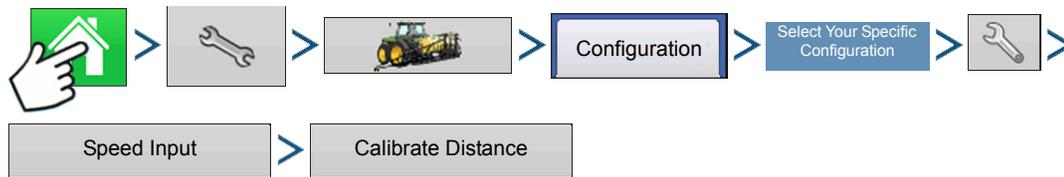
Press: Home button > Setup (wrench) button > Configuration (tractor) button > Configuration tab > your specific configuration > Setup (wrench) button > Speed Input button > Calibrate Distance
