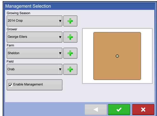
Enable Management    Un-checking Enable Management button will allow operator to continue to next screen without entering additional information on this screen (similar to Events Only mode).
