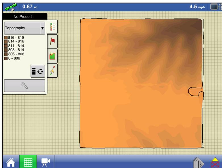
During collection of an elevation survey, points will be logged to the file every 3 meters. An onscreen visual will appear in the form of a single black dot every 30 meters.
