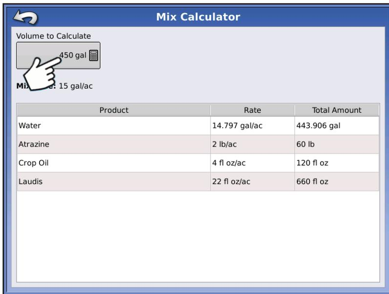
Press the Volume to Calculate button and input the total volume.
