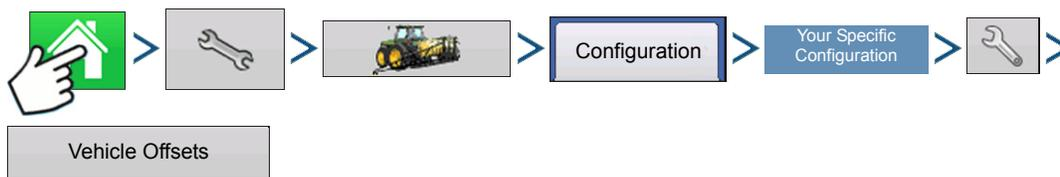
Press: Home button > Setup (wrench) button > Configuration (tractor) button > Configuration tab > your specific configuration > Setup (wrench) button > Vehicle Offsets button
