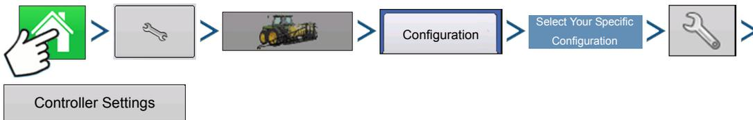
Press: Home button > Setup (wrench) button > Configuration (tractor) button > Configuration tab > select your specific configuration > Setup (wrench) button > Controller Settings button
