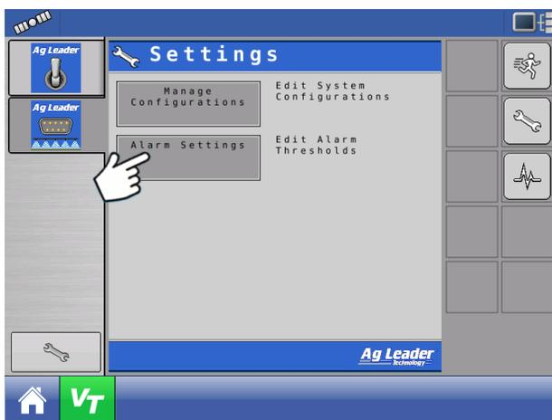
Press Alarm Settings button to edit alarm thresholds.
