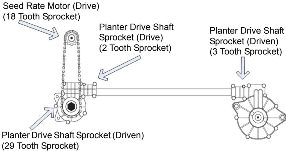
$$\frac{\text{Driven/Drive 1}}{\text{Drive 1}} \times \frac{\text{Driven/Drive 2}}{\text{Drive 2}} = \frac{\text{Driven}}{\text{Drive}}$$
