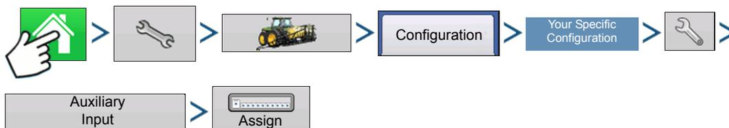
Press: Home button > Setup (wrench) button > Configuration (tractor) button > Configuration tab > your specific configuration > Setup (wrench) button > Auxiliary Input button > Assign button
