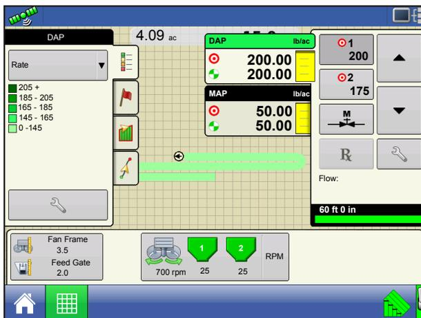
Conveyor rates for previously applied products can be found by first pressing the Settings button (A) which opens the Spreader Control screen.
