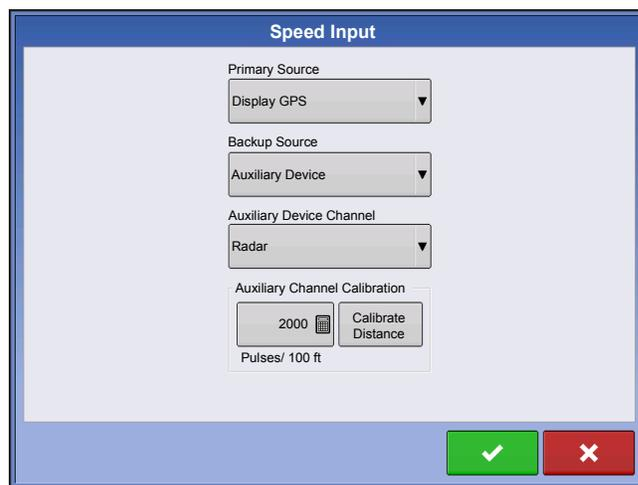
In most cases **GPS** is the primary speed source with **Radar** serving as backup. If you will be using **GPS** as the primary you will need to select a **Backup** source.
