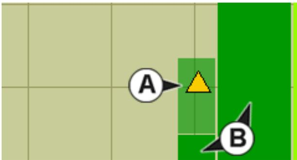
When the Map screen is running in a Zoom Detail view, **instantaneous coverage (A)** is shown automatically. However, there is a time lag between when grain enters the combine through the Header and is logged by the Flow Sensor in the Clean Grain Elevator. Because of this time lag, the instantaneous coverage is shown on the Map screen as a lighter color than **coverage that has been logged (B)** by the display.
