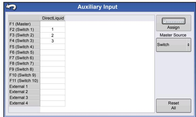
The **Assign** button, located at the upper right-hand corner of this screen, opens the Auxiliary Input Assignment screen, where you can assign functions to switches and external inputs. For more information, see [“Auxiliary Input Settings” on page 75](#).
