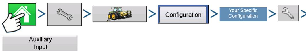
Press: Home button > Setup (wrench) button > Configuration (tractor) button > Configuration tab > your specific configuration > Setup (wrench) button > Auxiliary Input button
