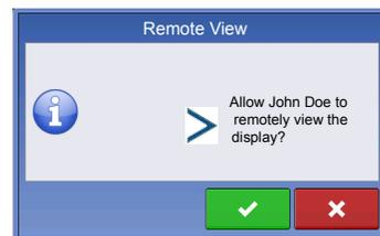
If buttons are grayed out then there isn't a remote support license tied to the AgFiniti account. Must enter Remote Support activation code at [www.AgFiniti.com](http://www.AgFiniti.com). See dealer for activation code.
