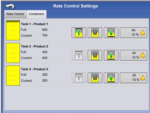
When filling or emptying container, use the Container Level portion of the Rate Control Settings screen to update the amount of product in the containers.
