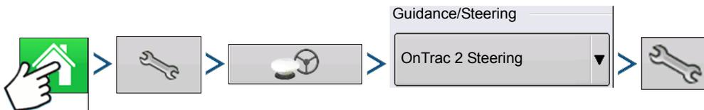
3. Press: Home button > Setup (wrench) button > GPS Guidance button > OnTrac2 Steering drop-down > Setup (wrench) button
