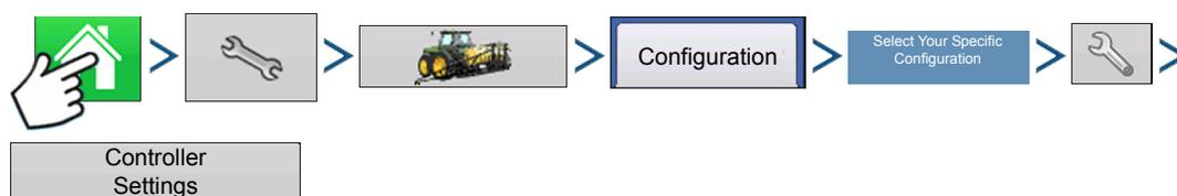
Press: Home button > Setup (wrench) button > Configuration (tractor) button > Configuration tab > your specific configuration > Setup (wrench) button > Controller Settings button
