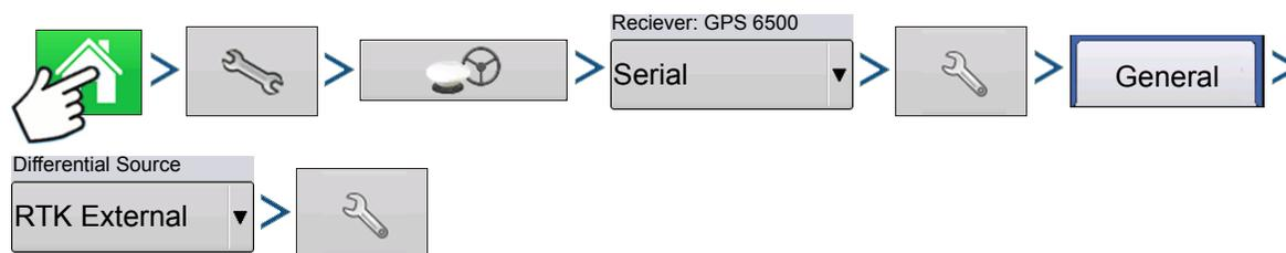
Press: Home button > Setup (wrench) button > GPS button > Serial (from Receiver drop-down box) > Receiver Setup (wrench) button > General tab > RTK External (from Differential Correction drop-down box) > Differential Source Setup (wrench) button
