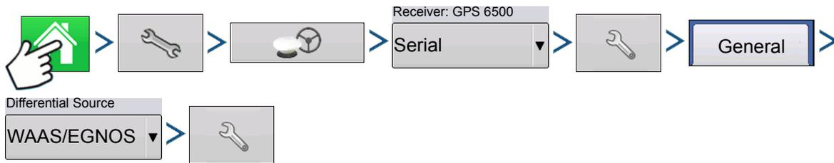
Press: Home button > Setup (wrench) button > GPS button > Serial (from Receiver drop-down box) > Receiver Setup (wrench) button > General tab > WAAS/EGNOS (from Differential Correction drop-down box) > Differential Source Setup (wrench) button
